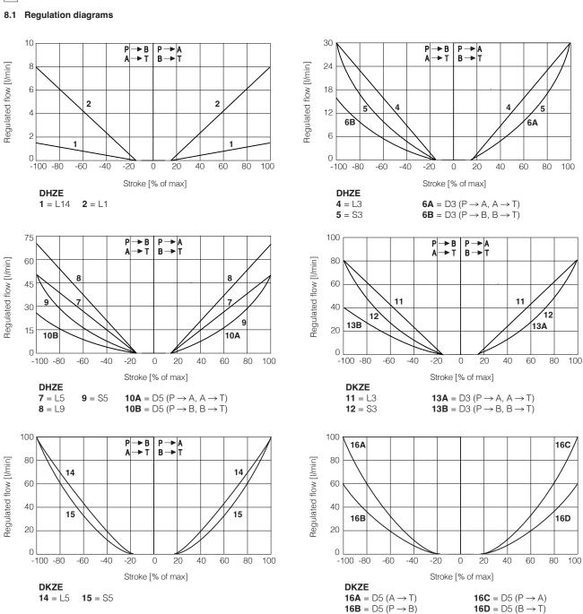
Note: Hydraulic configuration vs. reference signal for configuration 71 and 73 (standard and option /B)
